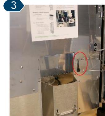
Expose the USB port by gently removing the rubber protective “stopper”.
