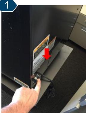
Power “OFF” the machine using the power switch located on the back left of the machine.
