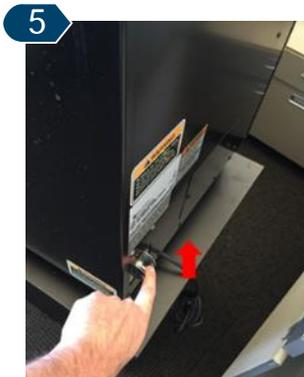
Power **"ON"** the machine using the power switch located on the back left of the machine. The software upload process will begin.
