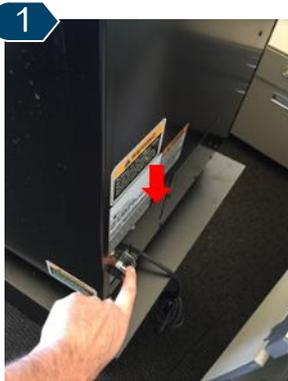
Power “OFF” the machine using the power switch located on the back left of the machine.
