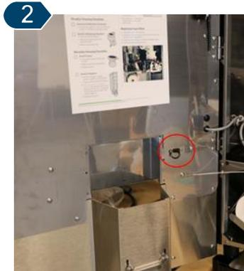
Open machine’s door and locate the rubber “stopper” covering the machine’s USB port. (lower right of machine door)
