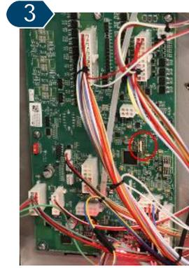
Locate the USB port located on the machine's internal board. Insert the USB drive with updated software into the USB port.
