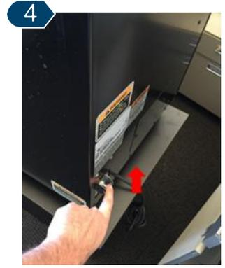
Power "**ON**" the machine using the power switch located on the back left of the machine. The software upload process will begin.
