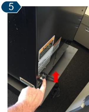
Power “ON” the machine using the power switch located on the back left of the machine.
