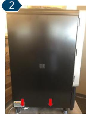
Remove machine's left side panel by **loosening** two ¼" screws located on the underside of the brewer. Place panel to the side.
