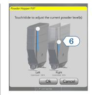
6) Close the door. Indicate the hopper fill level by pressing the onscreen fill line associated with the internal hopper.
