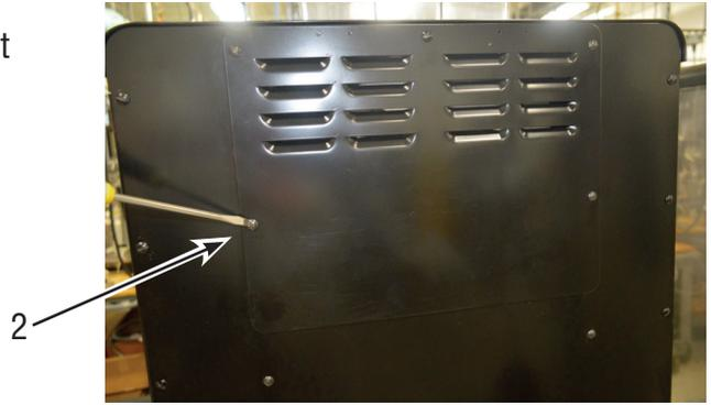
4. Use a 1/4" wrench to loosen (do not remove) the two (2) screws on the bottom (Figure 3) of the left side panel. Remove the panel and set it aside in a safe place and safe manner to avoid damage.
