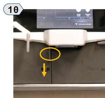
10 Once the software upload is complete, remove the USB drive from the USB port.
