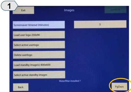
From the main Image screen, press **PgDwn** at the bottom of the screen until **LOAD BACKGROUND IMAGE** is visible.
