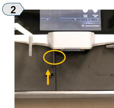
2 Remove the port's protective cover and insert the USB drive.
