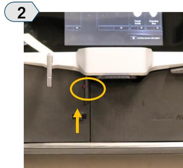
2 Remove the port's protective cover and insert the USB drive.
