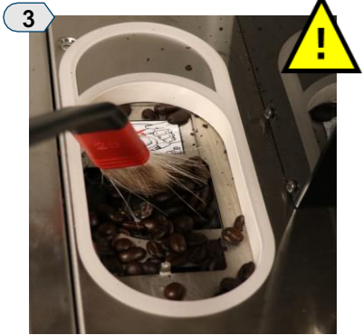
3 With a soft brush, brush any beans or bean fragments that may be keeping the hopper from sitting properly, away from around the grinder, then carefully remove.
