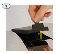
Unlock and open the cleaning tablet hopper located on top of the machine.
