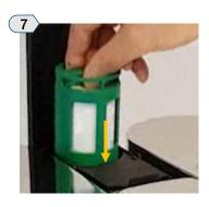
Slide the green holder back into the tablet hopper.
