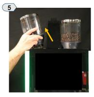
Gently lower the machine's display to allow clear access to the bean hoppers. Carefully lift the hoppers from the top of the machine.
