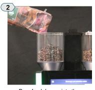
Pour fresh beans into the hopper and fill to desired level.
