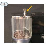
Unlock bean hopper lid using the provided key, then remove the lid.
