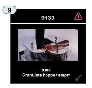
Press the ✓ on the screen to confirm that the hopper has been refilled.
