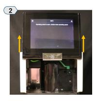
With two hands, gently pull the display upwards until it locks in the open position.
