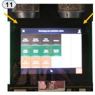
Lower the display then carefully push the top until it locks in place.
