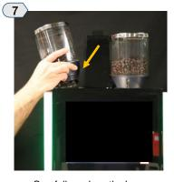
Carefully replace the bean hoppers over each grinder on top of the machine.
