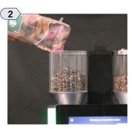
Pour fresh beans into the hopper and fill to desired level.
