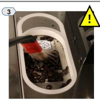
With a soft brush, brush any beans or bean fragments that may be keeping the hopper from sitting properly, away from around the grinder, then carefully remove.
