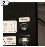
Turn ON the system pressure using the switch on the back of the unit
