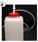
Attach the dispense end of the intake hose to the cleaning container. Push until the connectors "click" in place
