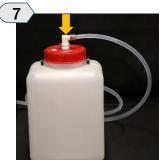
Attach the dispense end of the intake hose to the cleaning container. Push until the connectors "click" in place
