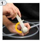
Open the inline filter adapter with the inline filter wrench by turning COUNTERCLOCKWISE.
