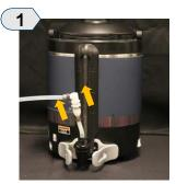
Disconnect the intake hose from the server by pressing the metal button on the server adapter
