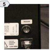
Turn ON the system pressure using the switch on the back of the unit
