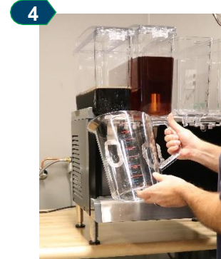
Drain product from all bowls by dispensing into a container. DISPOSE OR STORE UNUSED PRODUCT AS REQUIRED.
