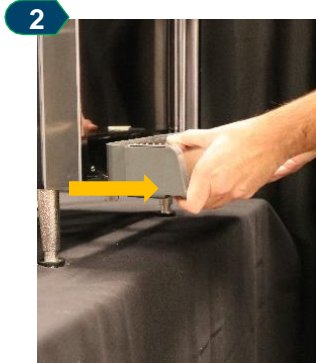
Remove drip tray from machine and drip tray cover from drip tray.
