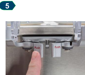
Press latches on the front of the machine until the bowls are released. Remove the bowls from the base of the machine
