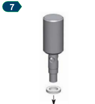
Remove O rings from dispense valves. BE CAREFUL NOT TO LOSE THE O-RING(S)
