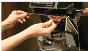
k) Close the main assembly door. Replace and lock the front panel above the drink spout, and reinsert grounds drawer.
