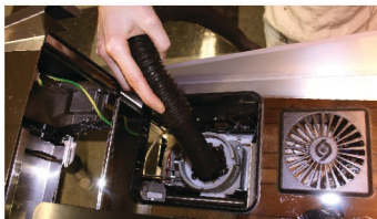
h) Vacuum the top of the machine and inside the bean hopper to remove any left over coffee bean remnants.
