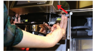
c) Pull the two latches on each side of the spout toward you to unlock the assembly door.
