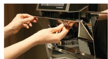
n) Close the main assembly door. Replace and lock the front panel above the drink spout, and reinsert grounds drawer.
