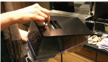
g) Unlock the hopper and remove the beans. Rinse with warm water and allow to completely dry.
