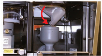
l) Re-open the powder outlet of the chocolate hopper by turning it counter clockwise.
