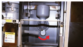
g) Remove the tube attached to the chocolate mixer. Unlock the mixer by turning the bayonet lock to the right and pulling the bowl out.
