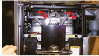
e) Turn locking pins on each hopper clockwise 90 degrees to unlock.
