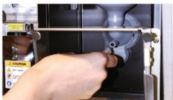
k) Reattach the tube by pinching the end and slowly working it back into the mixing bowl. Ensure it is well in place.
