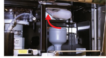
f) Close the powder outlet of the chocolate hopper by turning it clockwise.
