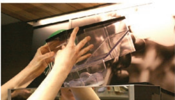
j) Replace bean hoppers when completely dry. NOTE: Bean hoppers must be completely empty when re-installed.
