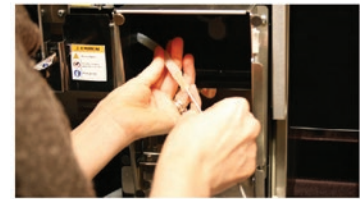
i) Clean the tube opening with a brush included with the machine.
