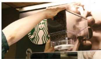
d) Lift and remove each bean hopper separately.
