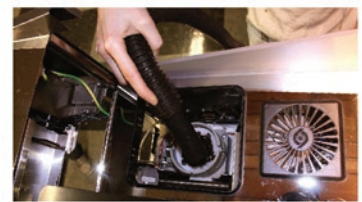
f) Vacuum the top of the machine and inside the bean hopper to remove any left over coffee bean remnants.
