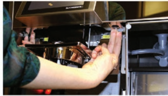
b) Pull the two latches on each side of the spout toward you to unlock the assembly. Open/lift main assembly door.
