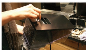
e) Unlock the hopper and remove the beans. Rinse with warm water and allow to completely dry.
