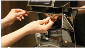
a) Unlock and remove front panel located above drink spout. Remove the grounds drawer.
