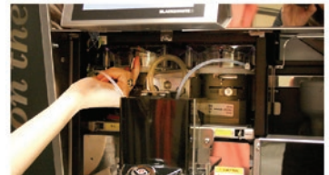
i) Turn locking pins on each hopper counter clockwise 90 degrees to lock. Close the main assembly door. Replace and lock the front panel above the drink spout, and reinsert grounds drawer.
