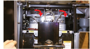
c) Turn locking pins on each hopper clockwise 90 degrees to unlock.
