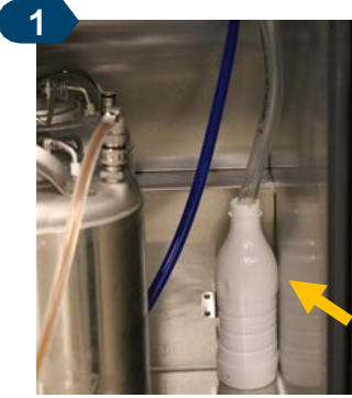
1 Unplug kegerator unit. Remove & empty drip tray drainage container. Disconnect and remove kegs.
