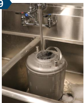
9 Using warm water, Thoroughly rinse the inside of the keg of all sanitizing solution
