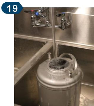
19 Fill keg (3 gal) with clean cool water . Replace the keg's lid and close tightly.
