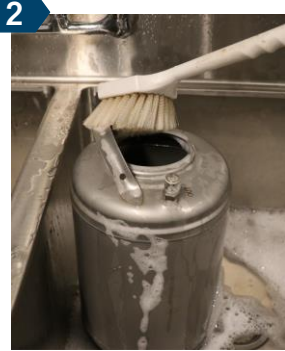
2 Using dish detergent, warm water and a soft brush, wash the inside and outside of the keg.
