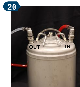
20 Connect the beverage & gas lines to the keg.. RED hose (gas) to "IN" CLEAR hose (beverage) to "OUT"
