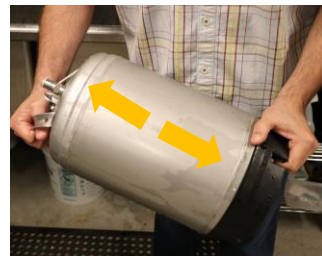
6 Shake or swirl the keg to cover all inside surfaces with sanitizing solution
