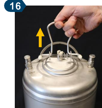
16 Once the pressure is released, it is safe to open the keg.
