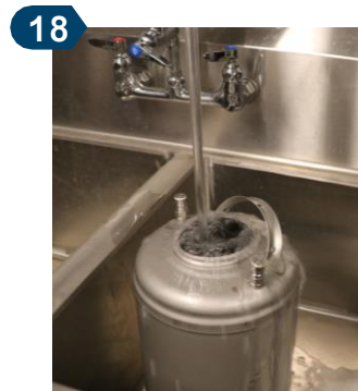
18 After 10min, THOROUGHLY rinse the inside of the keg of cleaning solution with clean water.
